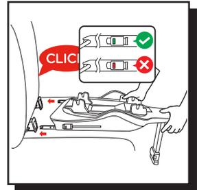
The ISOFIX connectors must stop in the ISOFIX anchor points of the car seat with an audible "click". Make sure the base remains firmly in place by trying to extract it from the ISOFIX connection guides. The GREEN safety indicator must be clearly visible on both ISOFIX release buttons.
