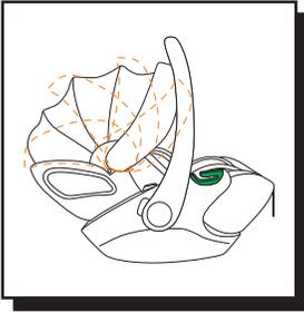
Unfold the sun canopy by pulling gradually on the plastic cover. To fold back, push the sun canopy back to its initial position.
