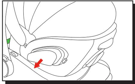
The «Linear Side-impact Protection» (L.S.P.) is built into the car seat. This system enhances the safety of your child in the event of a side crash. In order to achieve the best possible protective effect, unfold the L.S.P. (24) as far as possible towards the vehicle door closest to the car seat. To Release the L.S.P push the marked area (25) on the L.S.P. If it's not possible to completely unfold the L.S.P. with a closed vehicle door, you may as well use the infant car seat with a closed L.S.P.
