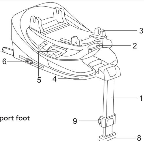
The base is equipped with a rotating mechanism for convenient installation of the infant carrier with a rotation towards the door. The platform rotation buttons are duplicated on both sides.
