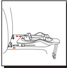
Release the ISOFIX connectors lock. Both clampings can be adjusted independently. Press both buttons simultaneously and remove the ISOFIX connectors from the base to the limit switch).
