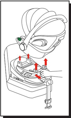
Pull the release button to unlock the Infant carrier and lift the Infant carrier with the handlebar. The base indicator will turn to RED.
