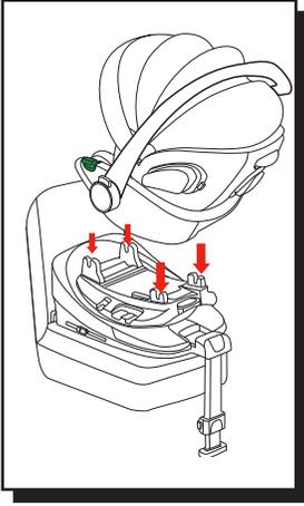
**IMPORTANT!** Make sure the surface of the base is clear from free objects and the child is secured with the integrated harness system in order to guarantee the correct installation of the base in the vehicle.
