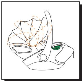
Unfold the sun canopy by pulling gradually on the plastic cover. To fold back, push the sun canopy back to its initial position.
