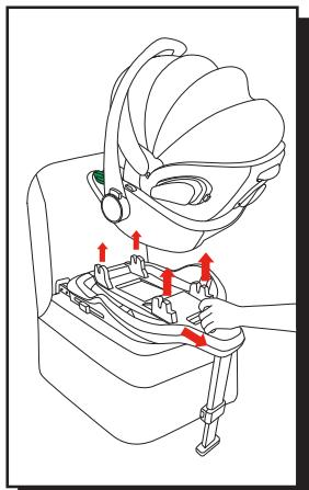
Pull the release button to unlock the Infant carrier and lift the Infant carrier with the handlebar. The base indicator will turn to RED.
