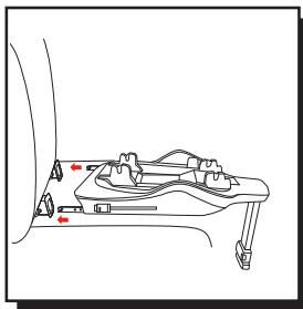
Release the ISOFIX connectors lock. Both clamping can be adjusted independently. Press both buttons simultaneously and remove the ISOFIX connectors from the base to the limit switch).
