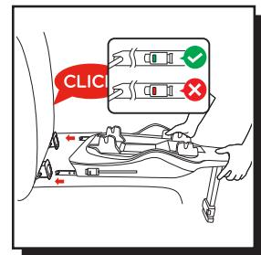
The ISOFIX connectors must stop in the ISOFIX anchor points of the car seat with an audible "click". Make sure the base remains firmly in place by trying to extract it from the ISOFIX connection guides. The GREEN safety indicator must be clearly visible on both ISOFIX release buttons.
