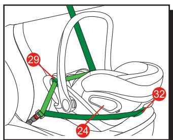
**! WARNING!** The infant car seat is not suitable for use with a two-point or lap vehicle seat belt. Securing with a two-point vehicle seat belt could result in serious injuries to the child in the event of an accident
