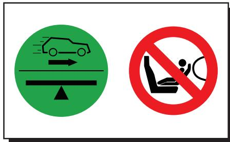
**NOTE!** The infant car seat is exclusively made for forward facing car seats, which are equipped with ISOFIX (Optionaly) or with a 3-point belt system according to UN R16 (see chapter «**Correct position in the vehicle**»).
