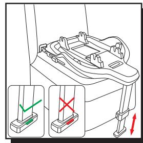
Make sure the support leg is fixed in a vertical position. Press the adjustment button: extract the support leg until it touches the vehicle floor. The support leg indicator on the foot will appear GREEN.
