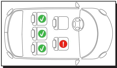
DO NOT place rear-facing baby car seat on front seat with active airbag, SERIOUS INJURY can occur.
